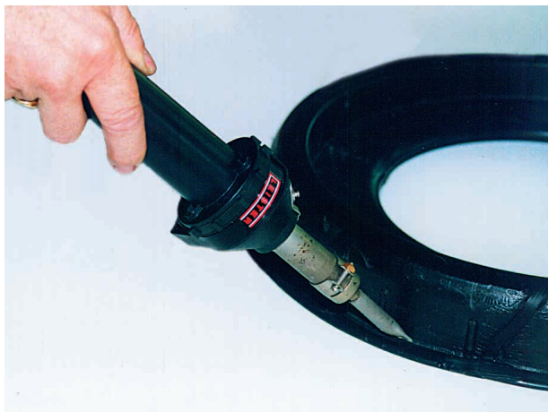
HOT-JET S being used for PE-HD tacking.
