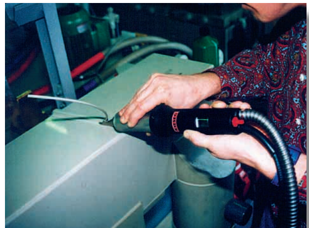
DIODE PID hot air tool with display and electronic control.
