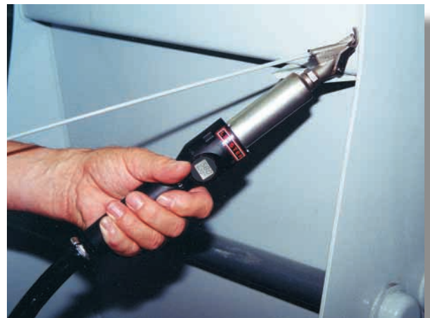
Welding PEN R with digital display for SET and ACTUAL value. The powerful welding tool.
