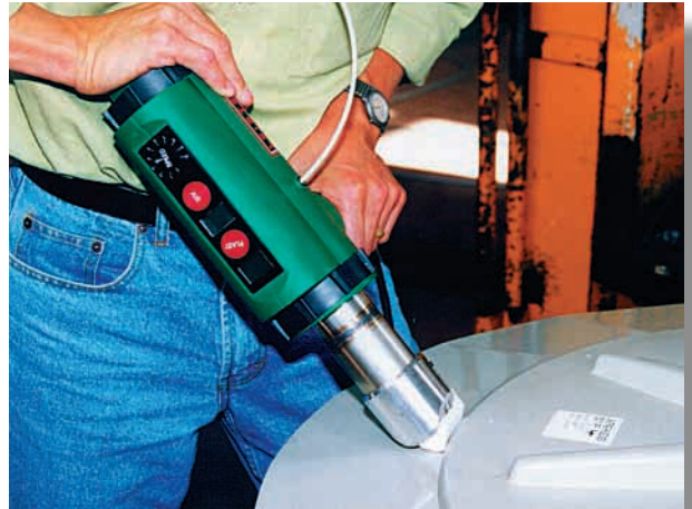
Weldmax Mini-Handextruder being used to weld PP
