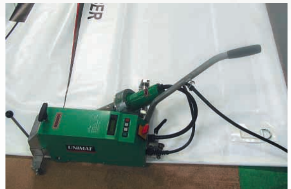
UNIMAT used for 40 mm flat hem weld of a coated cover. Welding speed up to 8.5 m/min. (28 ft/min).
