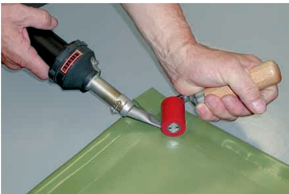
HOT-JET S with wide slot nozzle and pressure roller used for welding a billboard.
